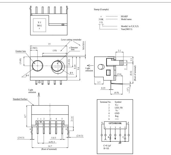
\* Position of the detector lens is not fixed because the sensor output is adjusted by moving the lens. Note 1. Unspecified tolerances shall be  $\pm$  0.3 mm.
